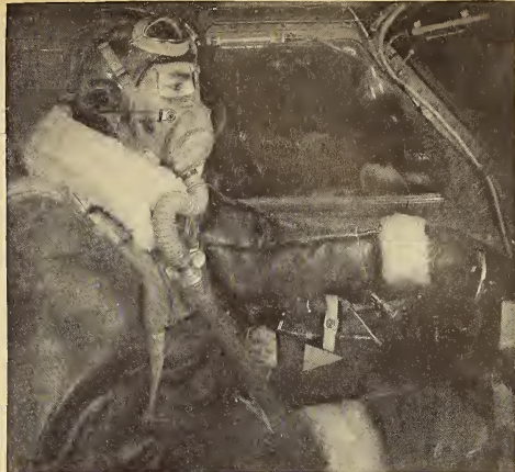
4. Above is pilot in a multi-place plane equipped with A-10 Demand Oxygen Mask. Similar precautions must be exercised in avoiding leaks with the revised A-10 as with this mask in order to insure proper regulator operation.
